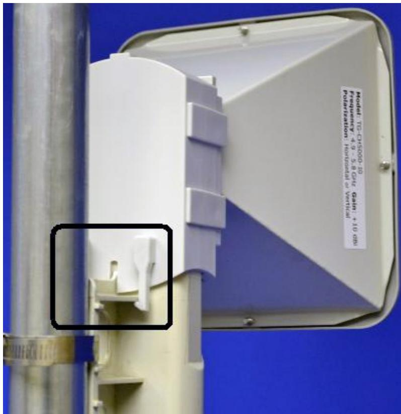
5. With the TG-CH5000-10 antenna installed, aim with the Canopy radio for peak signal.
